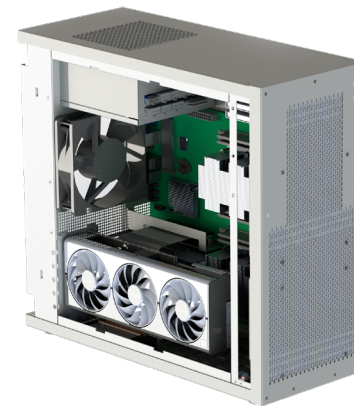
Nika 466533.506 System unit based on the NT Dragon 2C-3C5 «Manul-D» motherboard
